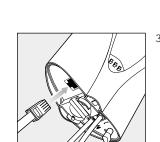
Connect the Remote Handset Lifter to your wireless system. Insert the AUX Plug into the large port marked AUX on the base of your wireless headset system (you will need to remove the Stand to access this port).\*
