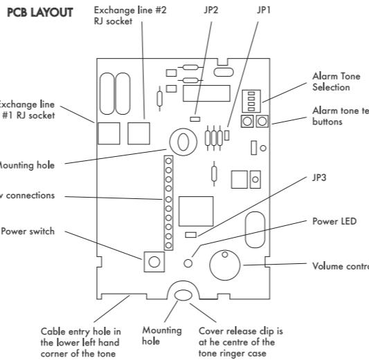
The exchange lines are connected using the "Line 1" and "Line 2" 6P6C RJ sockets. Only the two centre contacts (3 and 4) are used in each socket. All other connections are made via the 10 screw terminals - see the diagram on the previous page and refer to the relevant installation instructions for each type of device.
