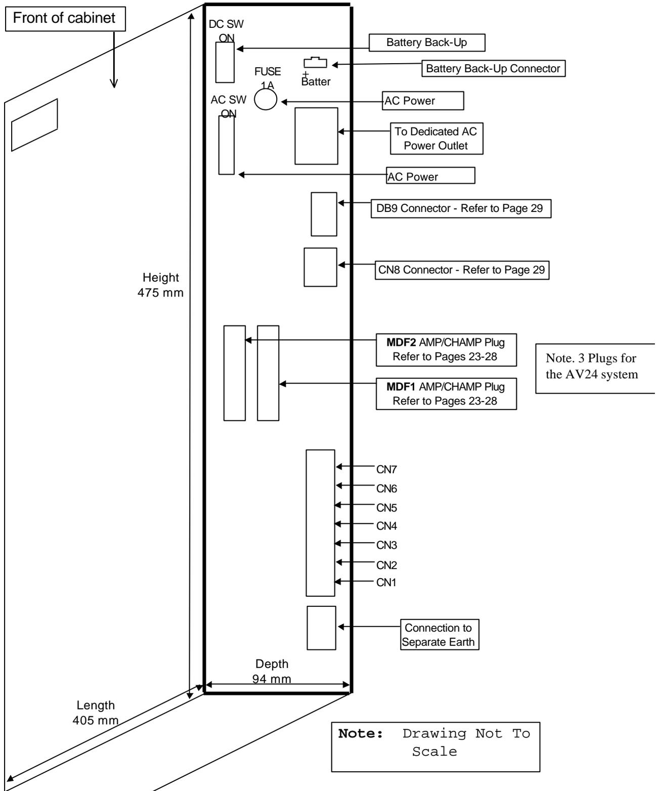
**Fig. 1-1. KSU Installation Layout**
