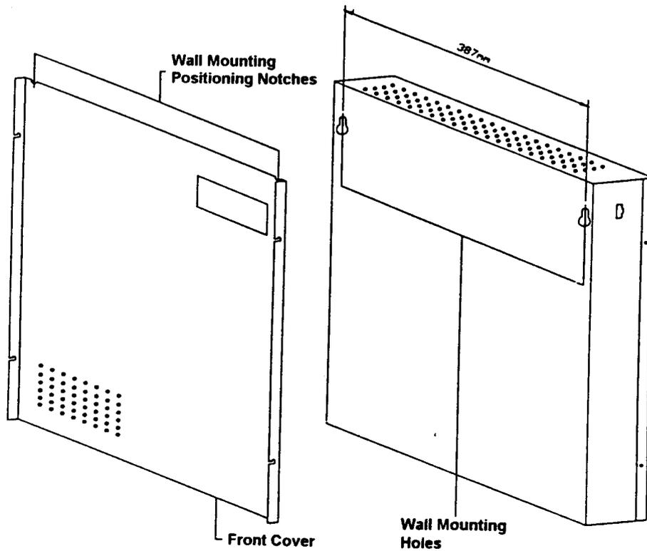
**Fig. 1-16. System Wall Mount Layout**
