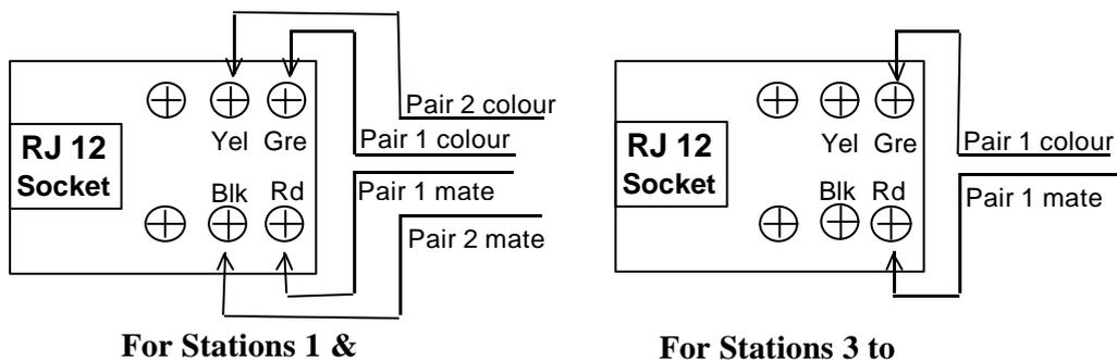
**Wiring diagram for socket
