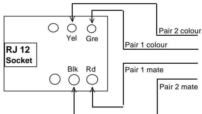
**Socket Wiring Diagram for Key Station**
