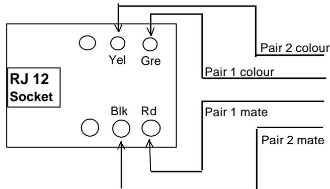
**Socket Wiring Diagram for Key Station**
