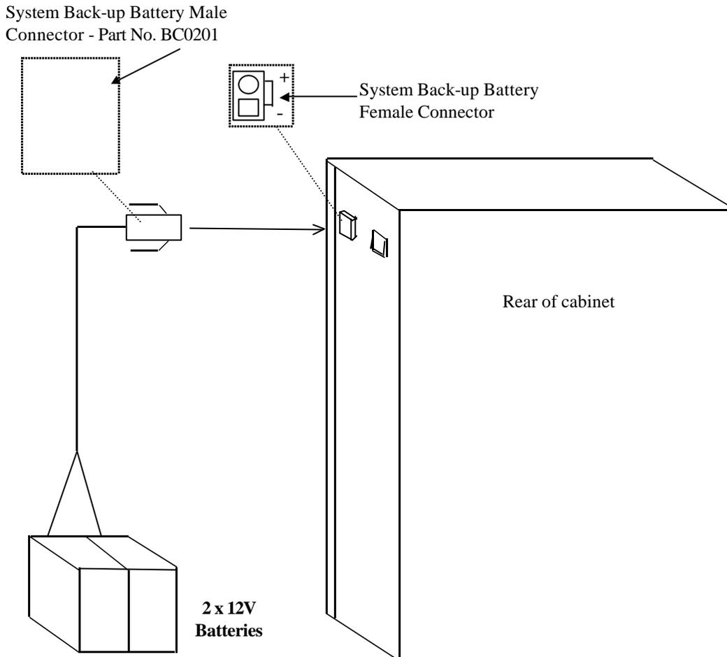
**Fig. 1-17. Battery Cabling Connection Layout**
