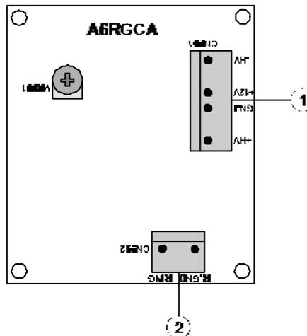
1. **CN901** : 4-Wire Connector. Connect to **[CN802]** on the **A6PWUA**.
