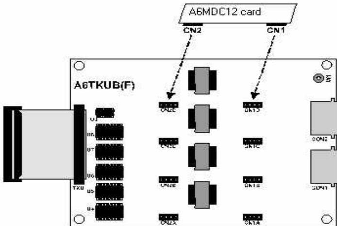
**Figure 20. Metering Pulse Detection Card Installation**
