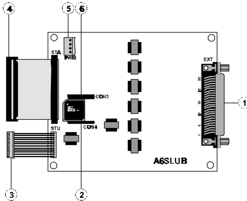
Figure 7. A6SLU 8 Port Single Line Station Card
