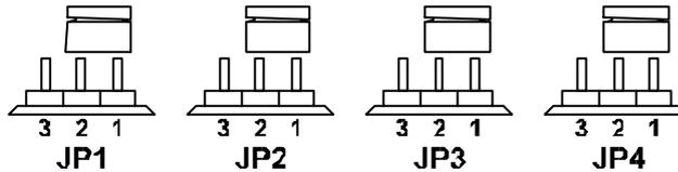
B. If the system's RS232 is connected to Serial Printer, ALL Jumpers 1-4 must have PIN2 and PIN3 SHORTED.
