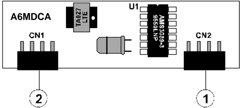
**Figure 12. A6MDC12 12KHz Metering Pulse Detection Card**
