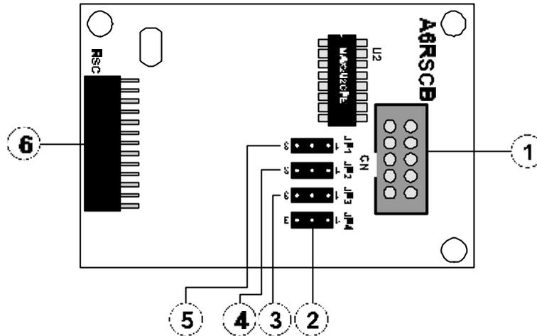
Figure 16. A6RSCB 2<sup>nd</sup> RS232 Interface Card
