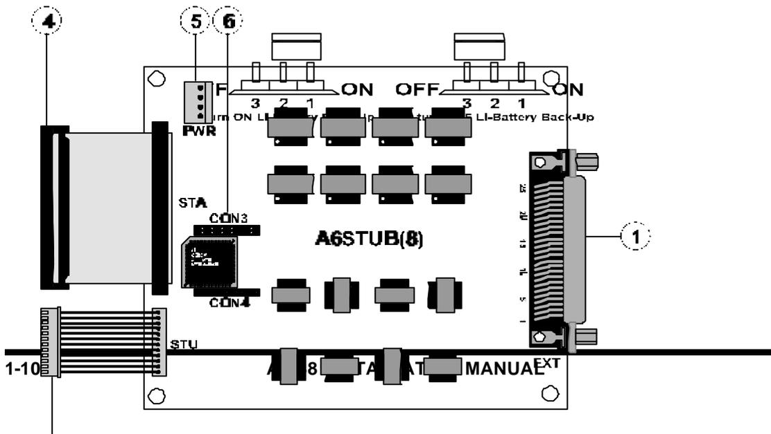
1. **EXT** : Amp Connector for Key Station Wiring
