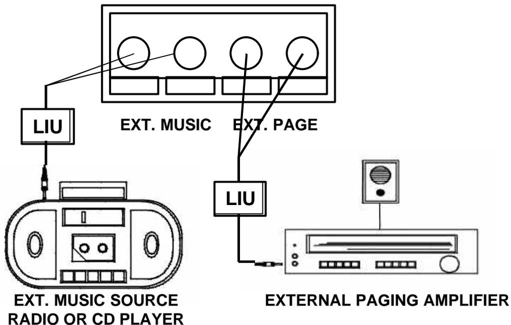
Figure 27. External Paging Equipment Wiring on A6MBUB
