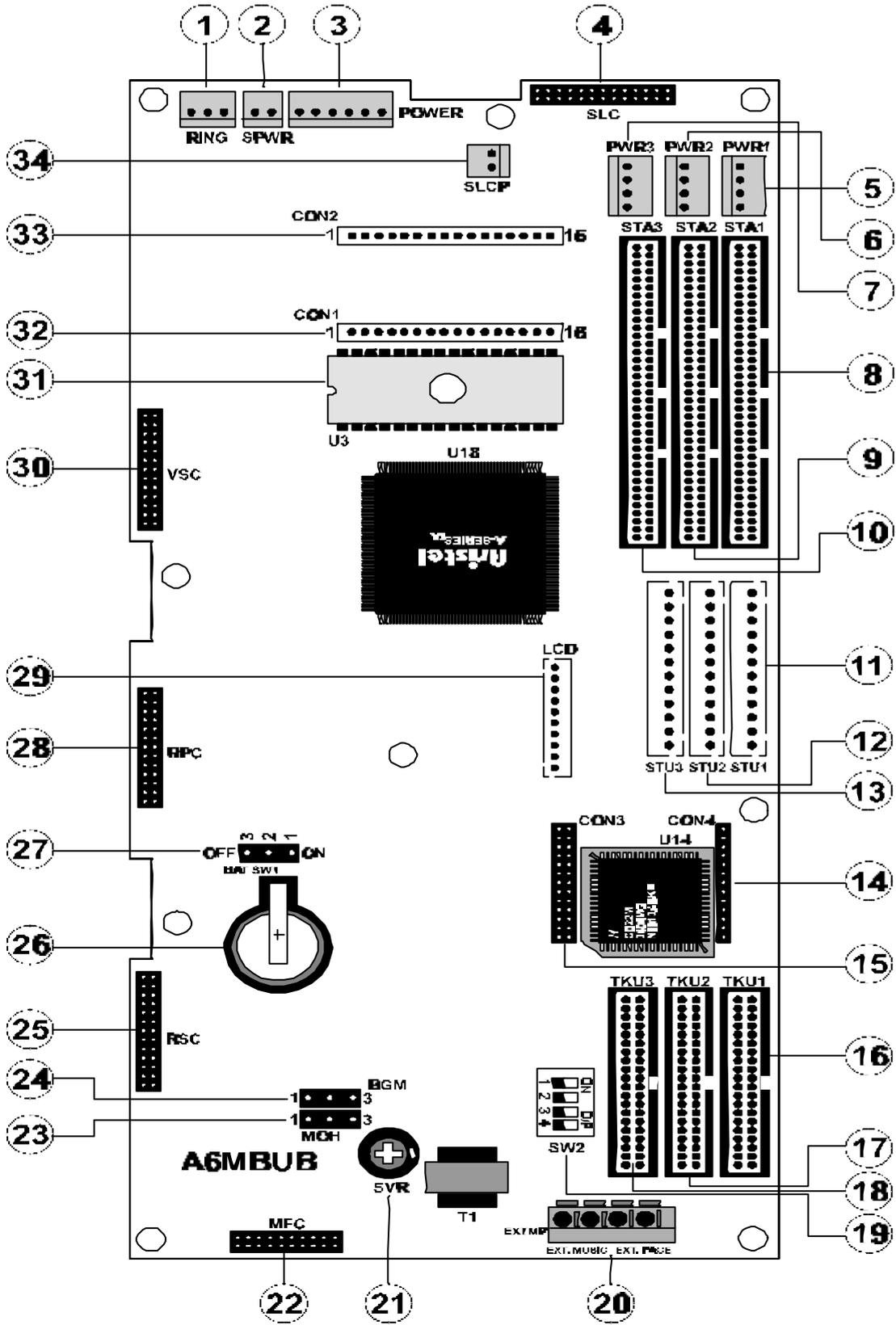
1. **RING** : 2-Wire Connector. Connect to **[CN902]** position on **A6RGC**.
