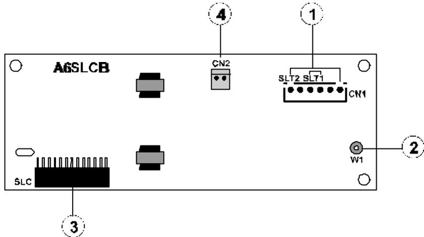
**Figure 8. A6SLC 2 Port Single Line Station Card**
