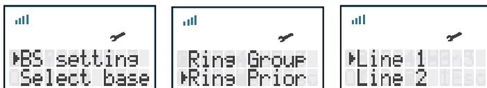
You can set external line access priority and assignment to a handset, the handset can then only use the assigned external line to make external calls. Each handset has choices of Alternative, Line 1 first, Line 2 first, Line 1 only, Line 2 only and No (No access to external line)
