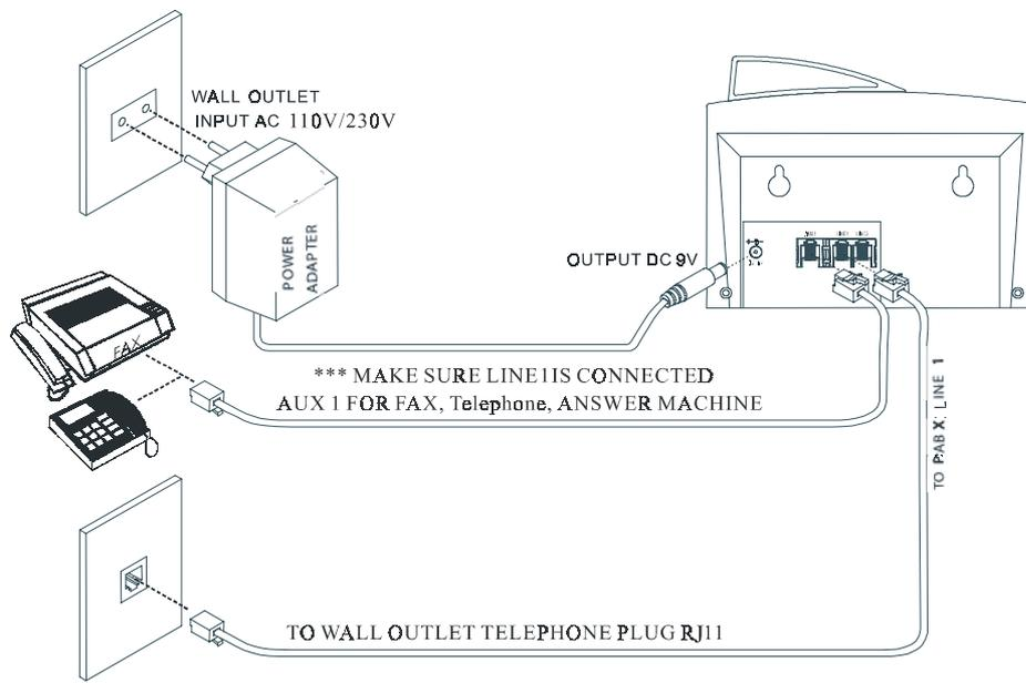
Plug one end of the adapter into the power outlet and the other end into the adapter jack on the bottom of the base.
