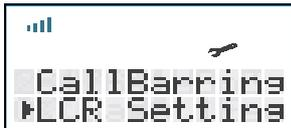
LCR can be programmed for:- **service provider** (digits to be inserted), **Code** (override code), **PABX code** (O/G access) and **Router** (On/Off).
