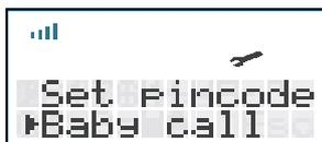
If you enable this function, the programmed number will be dialed automatically when any key is pressed. All other functions of the keypad will be disabled until Baby Call has been cancelled.
